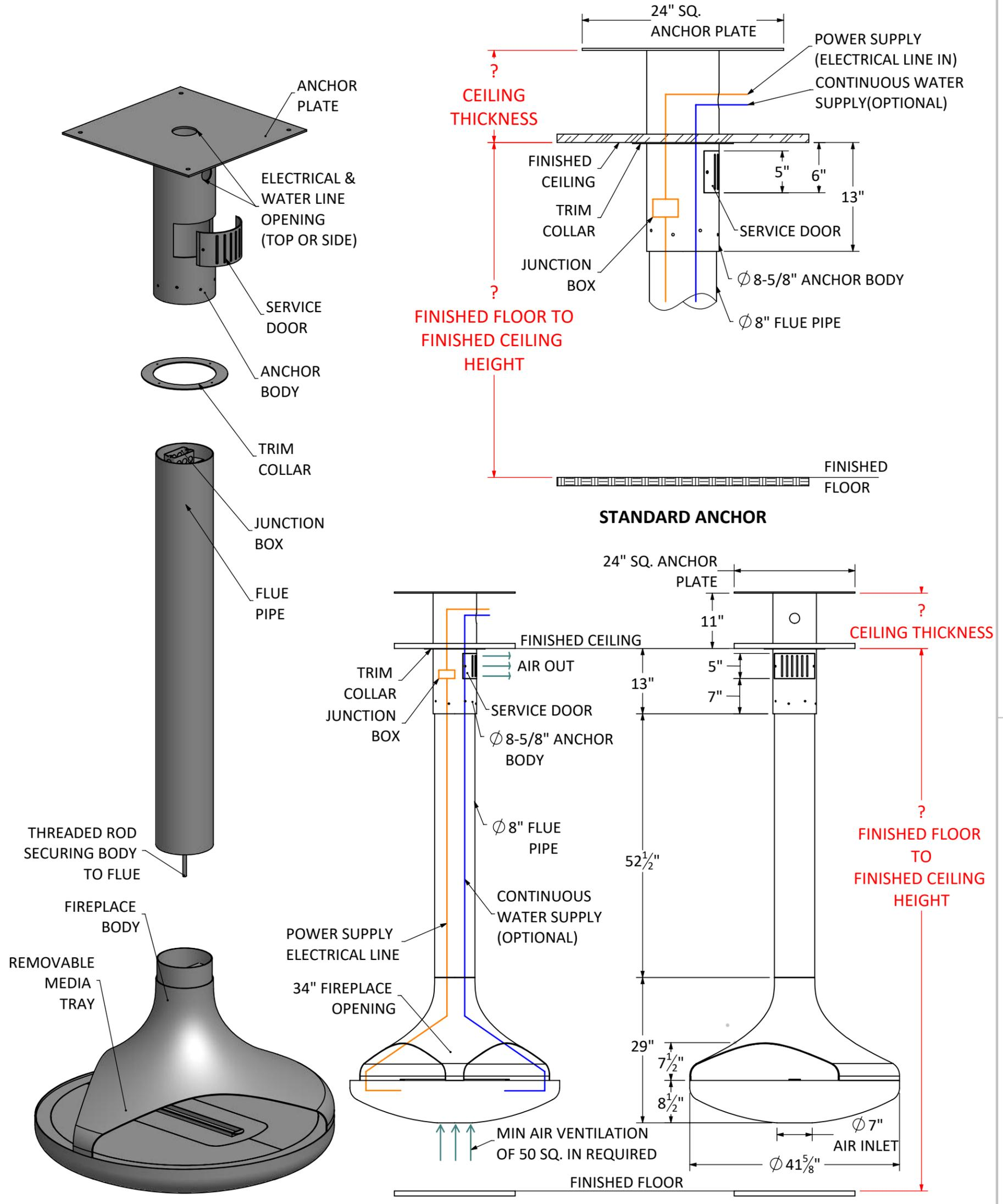
Shown with Standard 9 ft. Flat Ceiling Application with Vapor-Fire
