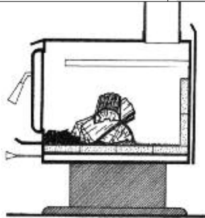
For a flash fire, use a few relatively small pieces of wood to "take the chill off." Load the wood loosely in a crisscross arrangement. Let the fire burn brightly until most of the solid wood is burned before reducing the air setting. Flash fires are effective in spring and fall when the heating load is modest. Using the flash fire technique, you can avoid smoldering fires.
