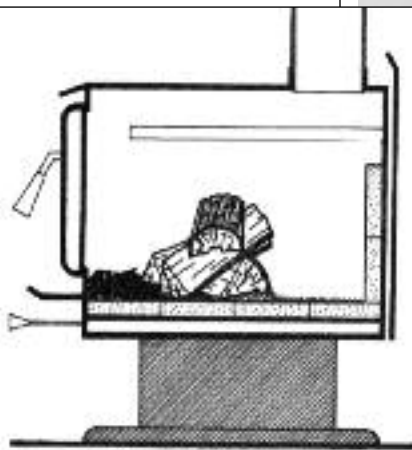
For a flash fire, use a few relatively small pieces of wood to "take the chill off." Load the wood loosely in a crisscross arrangement. Let the fire burn brightly until most of the solid wood is burned before reducing the air setting. Flash fires are effective in spring and fall when the heating load is modest. Using the flash fire technique, you can avoid smoldering fires.
