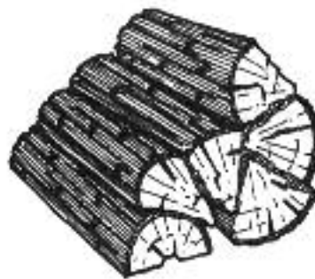
A compact fuel load is good for extended firing cycles
